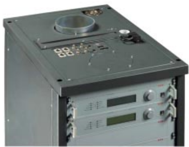
View of the chimney air inlet
